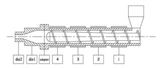
Type: screw: 45mm, L/D: 30, compression ratio 3:1
