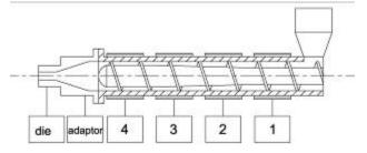
Type:45/25d(L/D=25) Screw compression ratio =3:1,
